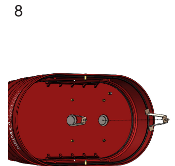
4 With the inlet blocked and motors running, transfer the holes using a 5/16" bit (3 holes each side).
